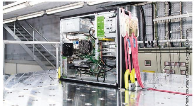
Vibration testing of a PC
