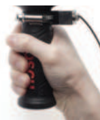
SV 150 Tri-Axial Hand-Arm Vibration MEMS Accelerometer
