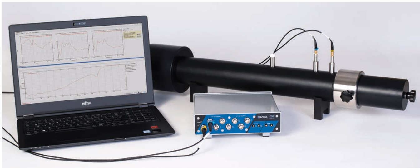
Impedance tube testing using m+p Analyzer software and m+p VibPilot front-end
