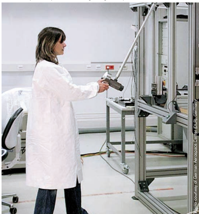
Shock Response Spectrum testing using an impact hammer
